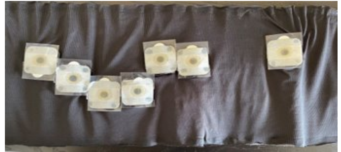
FIGURE 6: TORSO COMPRESSION STRAP INTERIOR SHOWING 7 ELECTRODE CONFIGURATION.
